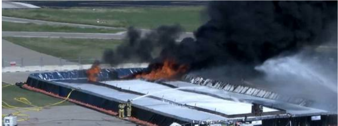
Fig 4.4 Large scale (40m) test CAF pouter application Virtual extinguishment. Note back up pouter not yet actuated and fire to right hand side outside the actual test pan
