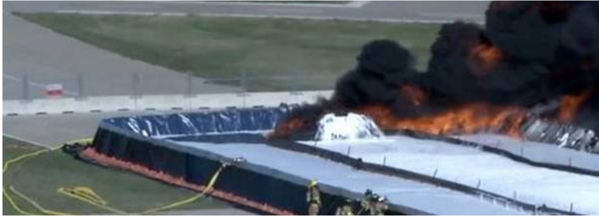
Back up pourer operating after extinguishment
