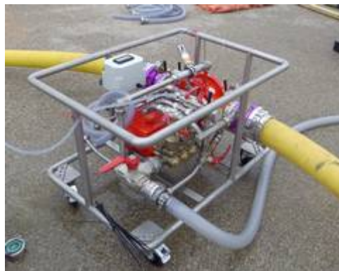
Fig 3.3. Water driven proportioner with calibrated flow meters package used during the tests
