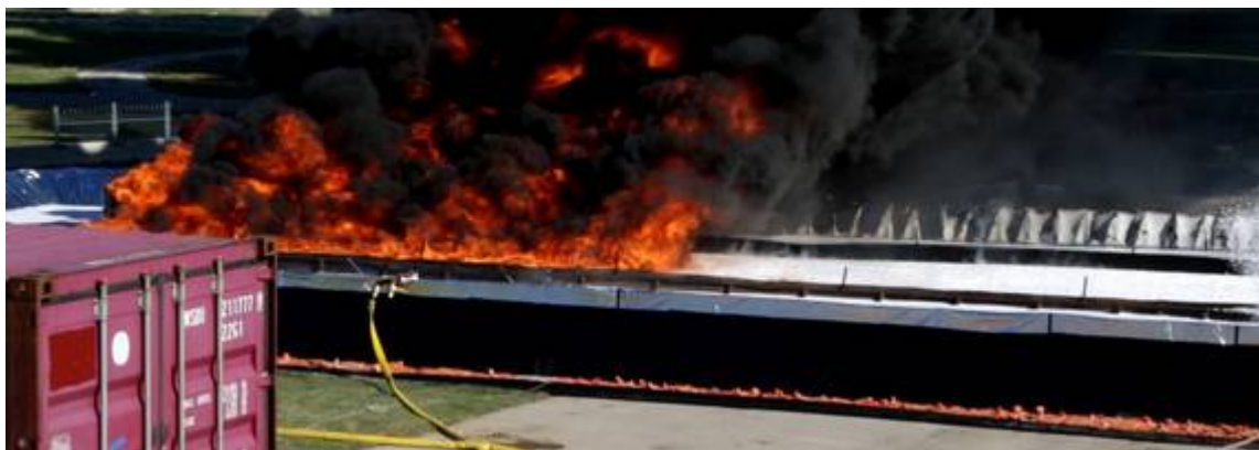
Fig 4.3 Large scale (40m) test CAF pourer application – extinguishment to ~30m
