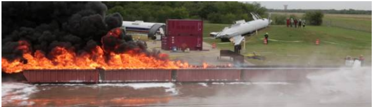
Fig 4.6 Large scale (30m) test being carried out – Conventional aspirated foam applied from right
