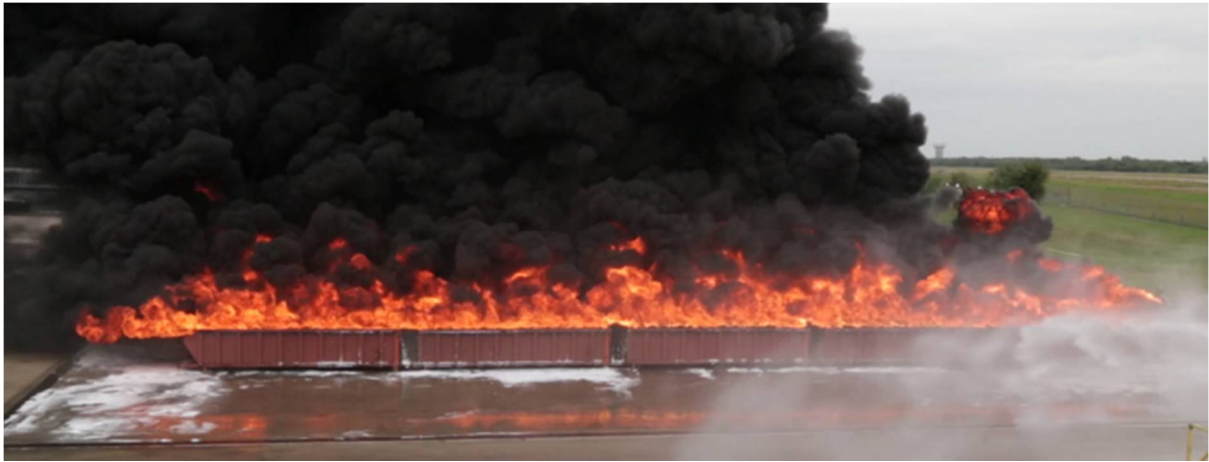
2) 30m length fire, Aspirating pourer application, 4lpm/m 2
