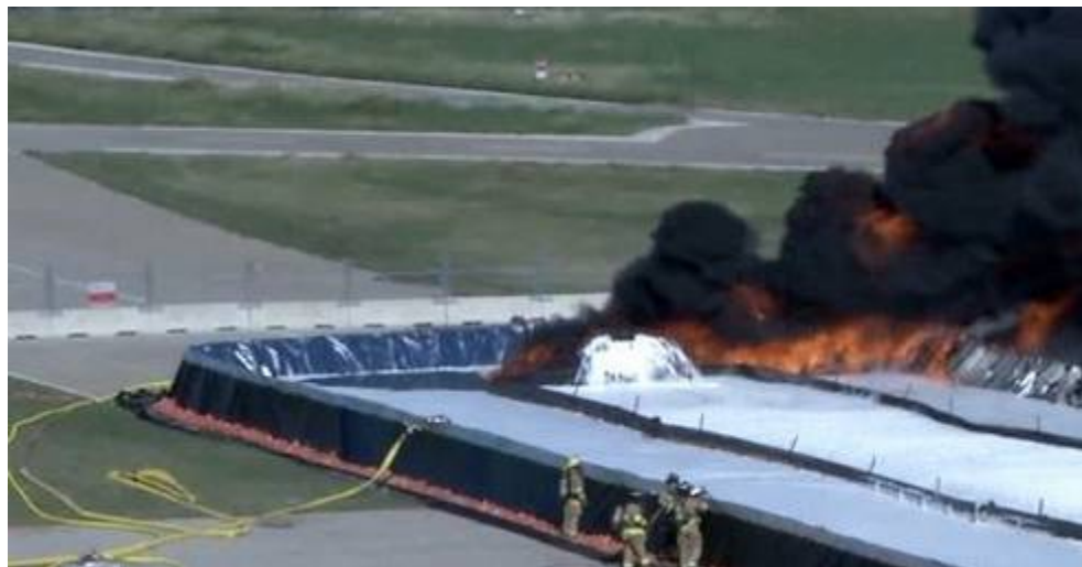
. Fig 4.5 Large scale (40m) test CAF pouter application. Full extinguishment in pan. Fire only in outer containment area and back up pouter actuated.
