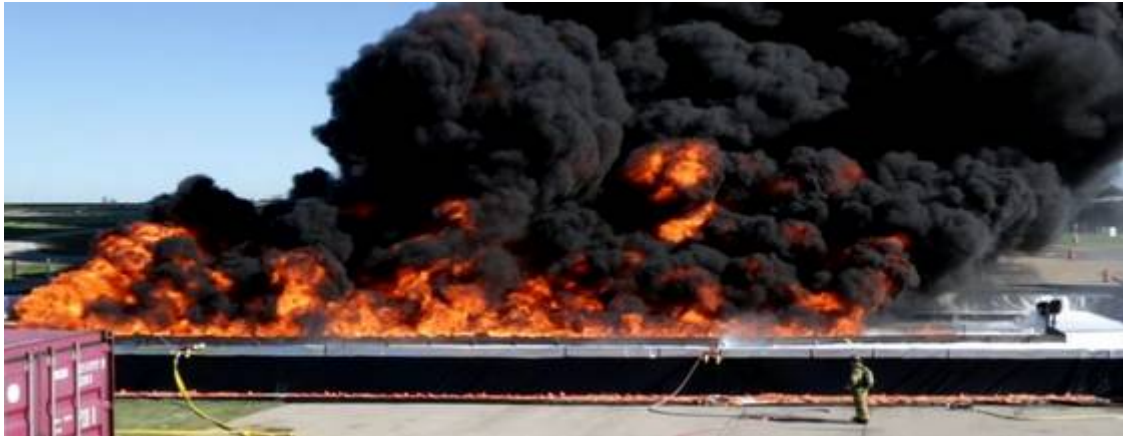
Fig 4.2 Large scale test (40m) being carried out – CAF foam applied from right
