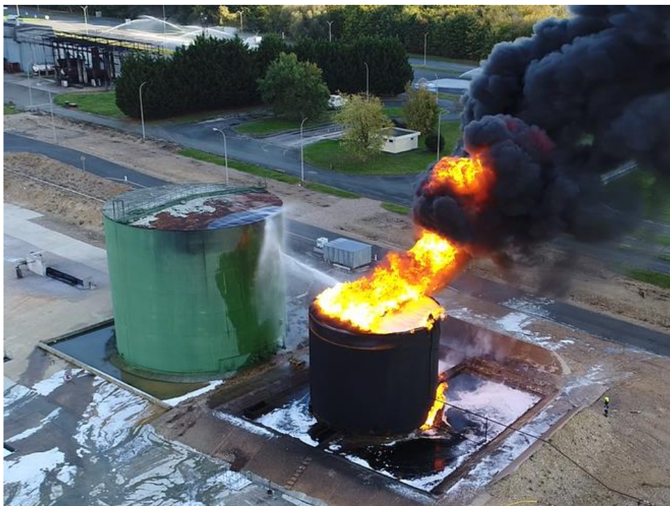
Fig. 2 Control beginning as foam flows across tank from pourer
