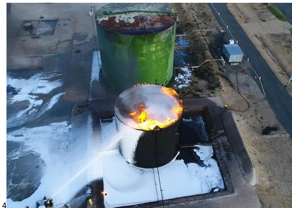
Fig. 6 Note edge sealing on edge near application device as new foam pushes foam against edge
