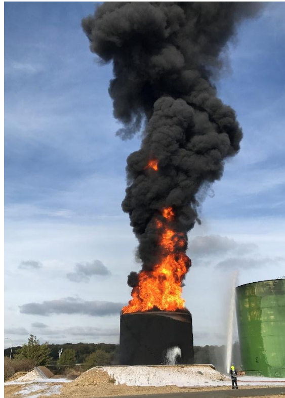
Fig 5.9. Cooling of adjacent tank during tests (note different wind conditions affecting flame drag)
