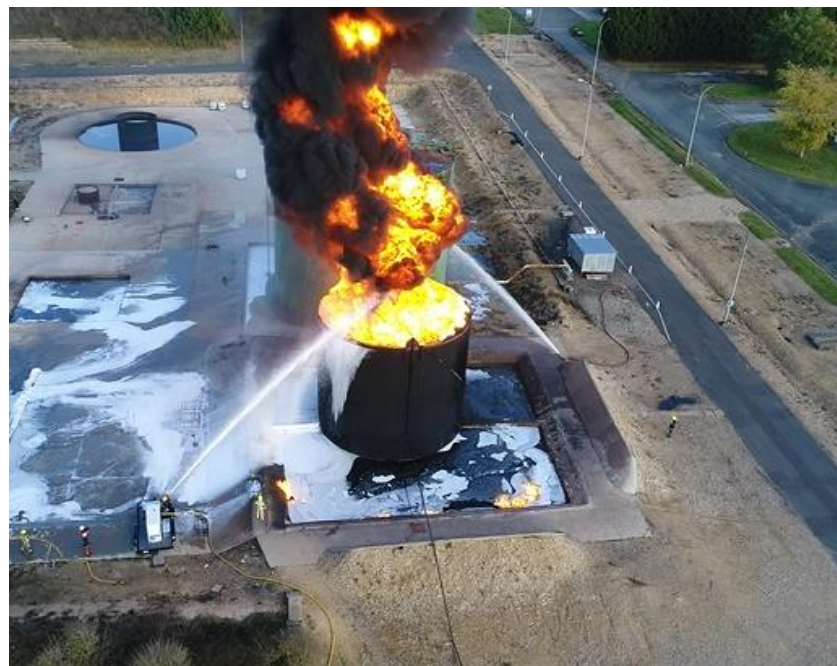
Fig. 2 CAF application into tank
