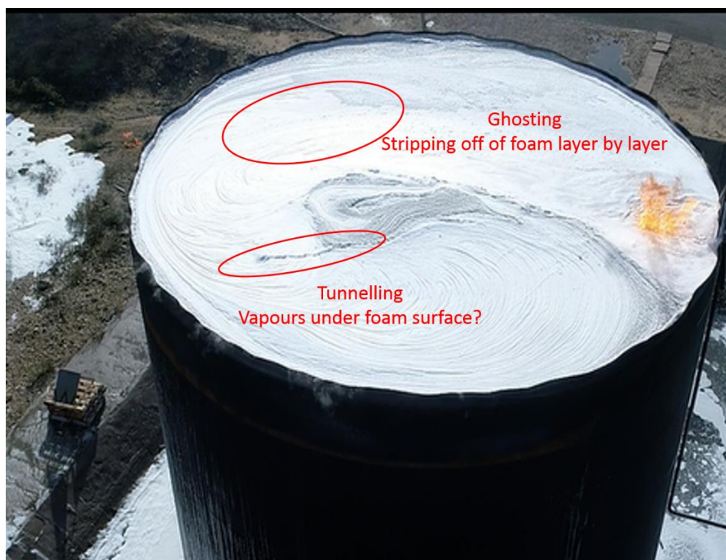
Fig 14. Tunnelling and Ghosting destroying layers of foam bubbles and impact area still ignited. Note impact area would probably be extinguished if foam application stopped but this is not a preferred policy. It is much better if full extinguishment is achieved with foam application still running.
