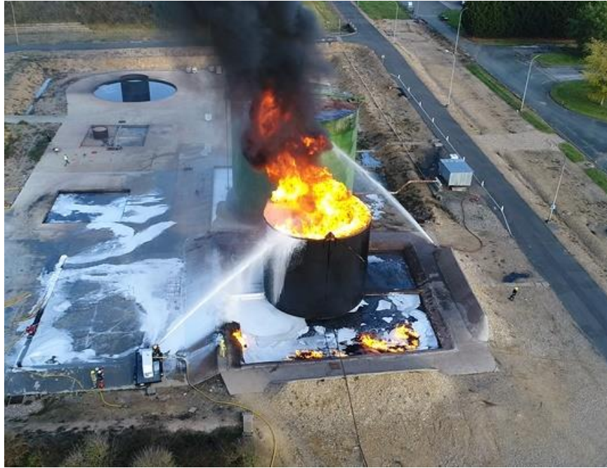
Fig. 3 Control beginning as foam blanket starts to form
