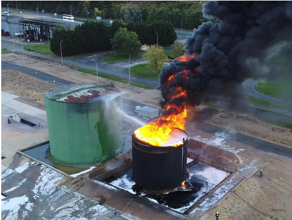
Fig. 3 Better quality foam seals edges as it travels across tank Extinguishment also achieved at impact area
