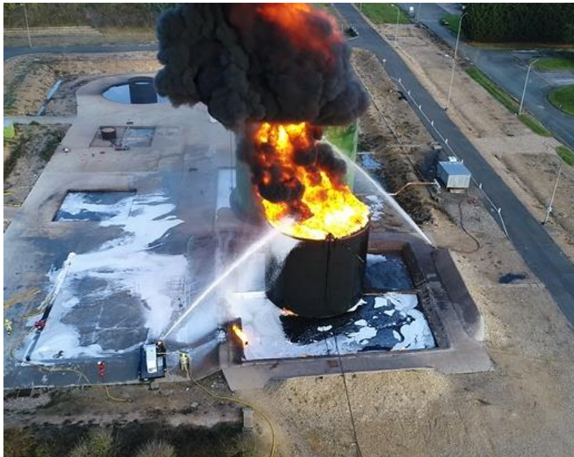
Fig. 1 CAF application into tank
