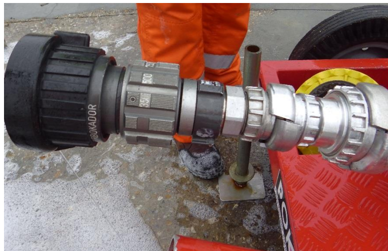
Figure 5.2. Non-aspirated POK monitor used during Phase 2 tests
