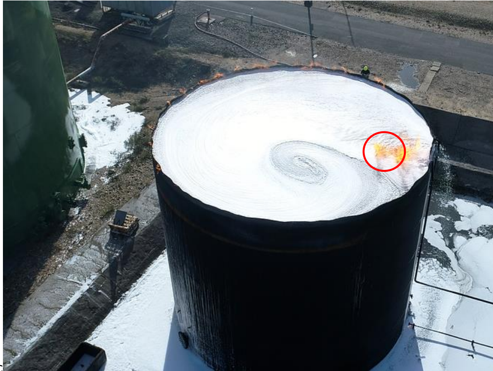
Fig 13. Edge flickers reduced in size but impact area continues to burn Note also “old foam” swirl
