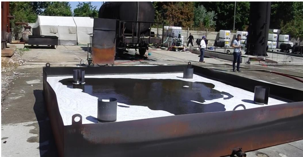
Figure 4.4. Large bund test pan with obstacles
