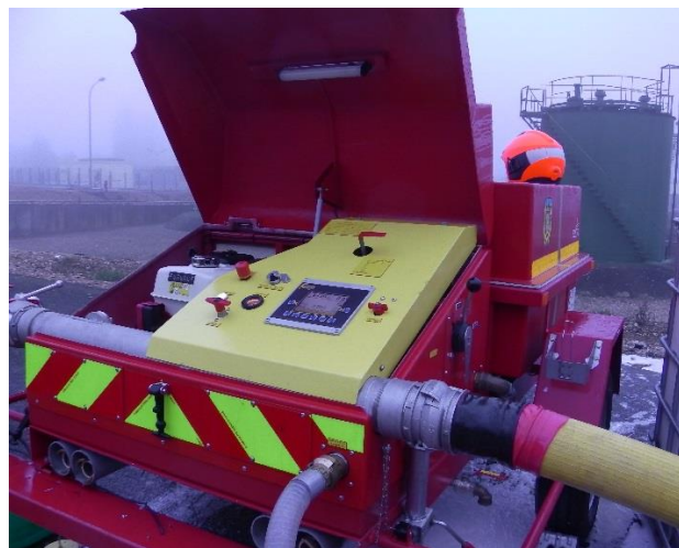
Figure 5.6. CTD "metered flow/controlled pump" proportioner unit used during Phase 2 Tests
