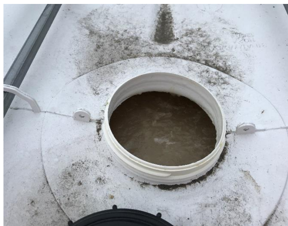
Fig 5.7. Foam in IBC seeming to form a ‘glossy skin’ during storage between test phases
