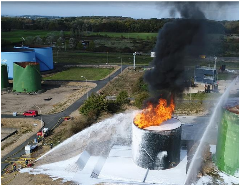
Fig. 4. Further build-up of foam blanket
