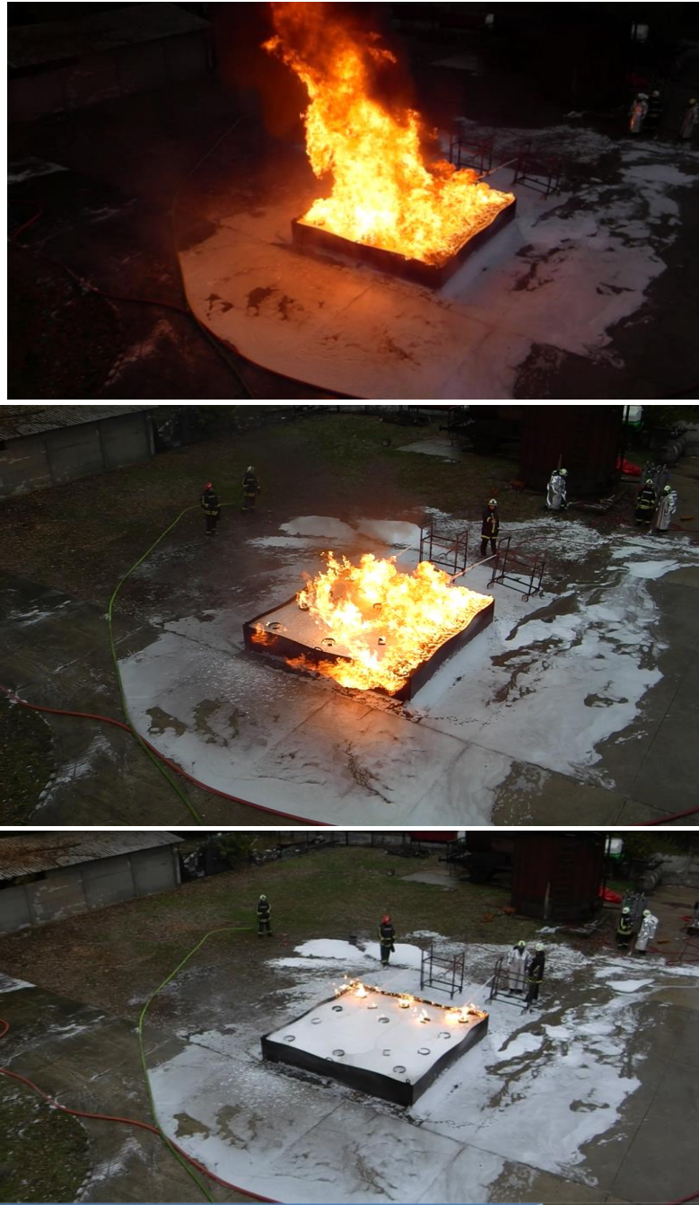
Figure 3.2. Sequence of fire test using monitor application. Note two nozzles being used for full bund fire (very low application rate)
